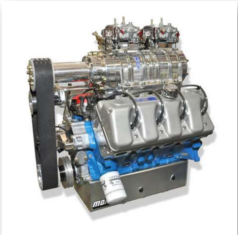
Though a variety of engine capacities can be specified, from 429 to 600cu in, the most popular displacement has proven to be 520cu in. And so it is with the blower version. By using a 429 passenger car block with a .030in overbore (4.390in) and a 4.300in stroke ensures engine parts are readily available, making this the most cost-effective unit to build.
