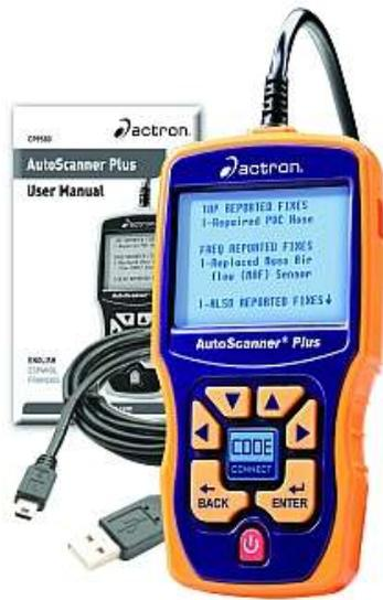
Compatible with 1996 and newer vehicles, AutoScanner Plus (Product Number CP9580) is a trilingual OBDII, CAN and ABS Scan Tool delivering live engine data in English, Spanish and French. This new generation scan tool can also record, graph and play back real time data as well as read and erase generic and manufacturer specific trouble codes.
