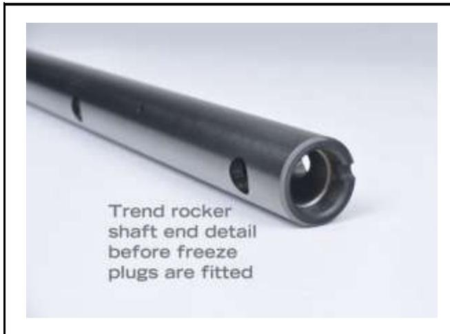
Created to overcome deflection and to improve valve-train stability when used in conjunction with high-performance camshafts and valve train, Trend produces this new shaft from thick-wall 4130 chrome molybdenum, subjects it to two heat treatments-through-hardening and nitriding-and finally applies a DLC (diamond-like coating).
