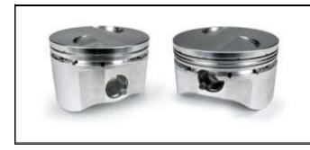
Easily recognized by its minimal ring pack, the benefits of the two-ring piston are lighter weight, less drag, and resulting higher rpm. The undesirable effects of drag are further reduced by the adoption of a thin 1.2mm top ring and a 3.0mm oil control ring. The second ring of the three-ring piston measures a slim1.5mm. All ring sets are by Total Seal.
