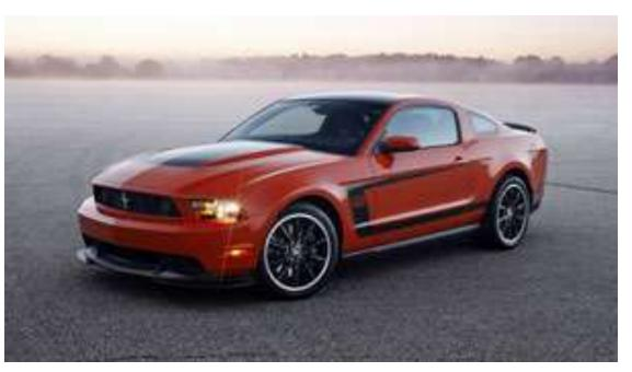
proven - on the Boss 302R race car. The front splitter is designed to function at high speeds by efficiently managing the air under and around the car. It helps to reduce underbody drag and front end lift while more effectively forcing air through the Boss-specific cooling system. At the rear of the car, the spoiler was chosen to complement the front aero treatment and minimize overall drag.
