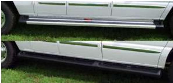
Owens' new Thermoplastic Polyolefin (TPO) molded board is available in both 100" and 120" and comes with a full-length, galvanized steel support which provides durability and serviceability. These TranSender boards have a tread design embedded in the TPO, providing secure footing year around with flair.
