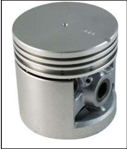
The L2037 pistons from Egge have a 7.0:1 compression ratio at 2.0625" compression height with a 3.5625" standard bore and uses two 3/32" compression rings and one 3/16" oil ring. The piston has a flat head design with a full skirt featuring a steel supported pin boss and a .865" wrist pin.
