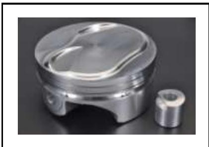
Compared with the removal of the secure yet unwieldy spiral locks or round wire locks, changing buttons is remarkably convenient. In addition, on pistons where the pin bores intercept the oil control ring groove, the buttons prevent the expander in the oil control ring from distorting around the half moon openings in the back of the groove, a deficiency more prevalent in power adder engines.
