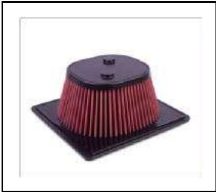
AIRAID engineers have been hard at work designing one of their most impressive filters yet. By utilizing a cone shaped filter to mesh with a flat panel base they added 35% More Surface Area to the filter inside the stock air box. More surface area translates into more airflow without compromising filtration. This increased airflow allows the engine to breathe better which increases horsepower, torque and overall fuel economy.
