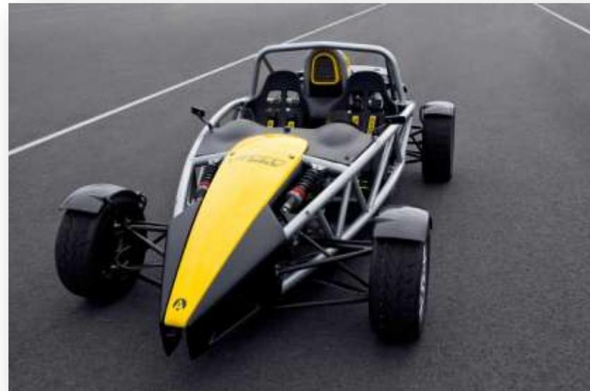
fact, it doesn't even have any conventional body panels—the driver and single passenger are exposed to the elements through an exposed tube frame.
