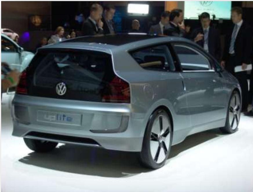
curb weight. Volkswagen made extensive use of aluminum; passenger compartment floors, trunk floor, engine compartment and firewall, and front windshield crossmember. Realizing that every ounce counts, Volkswagen substituted a carbon fiber composite for more traditional roof materials and cut more than 2 pounds. Sprinkled into the mix are a number of components made from magnesium.
